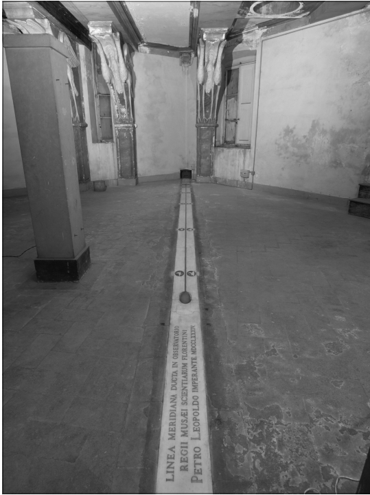
Fig. 3 (left). The Meridian Line, length 7.775m, with the winter solstice ellipse in the centre of the picture and the shutter and gnomonic hole near the ceiling at the top of the picture.
