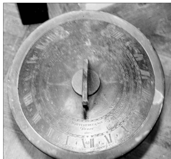
Fig. 17. One of the more complicated John Whitehurst dials, including an EoT scale, in Derby Museum.
