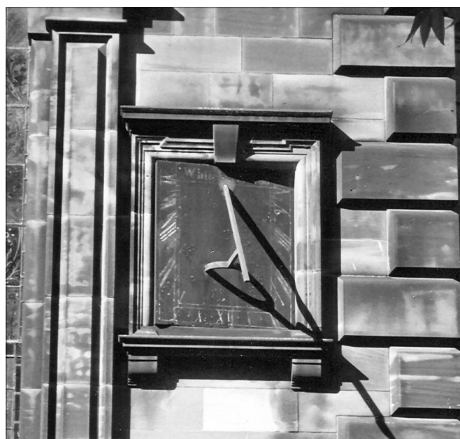
Fig. 8. The vertical south dial at St Modwen, Burton-upon-Trent, canted slightly to the east.
